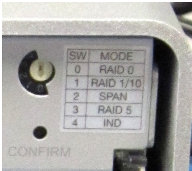
Fig. 11 A RAID configurable switch.
