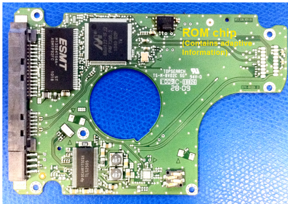
Fig. 4 A PCB showing a ROM chip .
