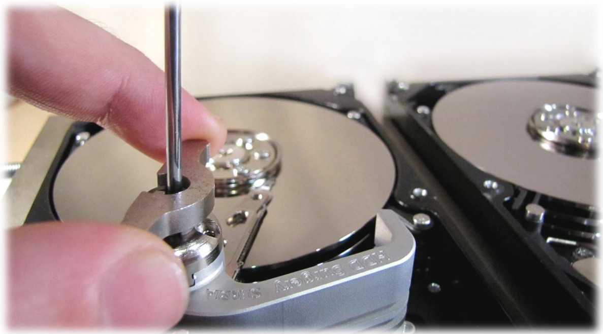
Picture 9 (removing the tool, using the assisting tool)
