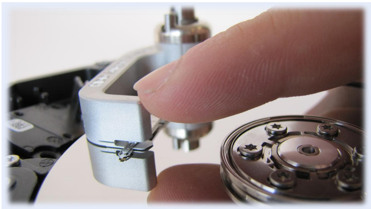
Picture 4. (moving secured tool with heads outside of platters area)
