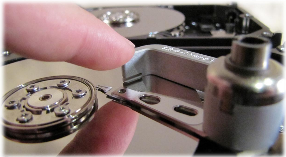
Picture 8. (returning the tool outside of platters)
