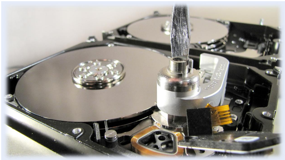
Picture 6. (mounting the heads on a patient drive)
