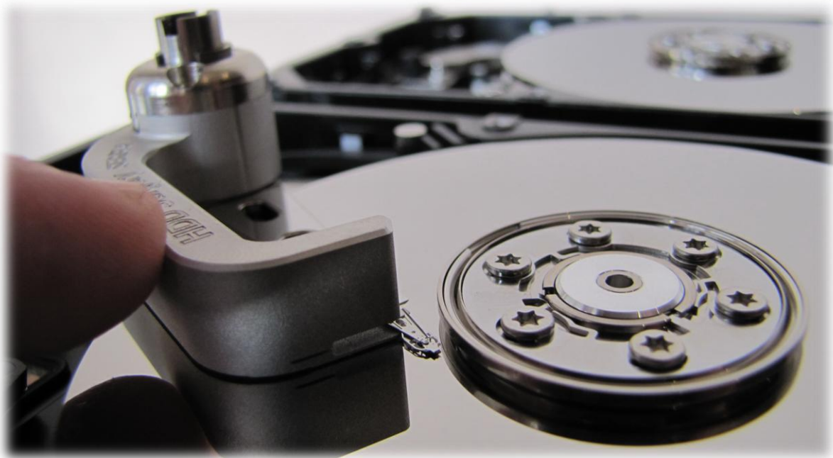
Picture 2. (lifting the heads)
