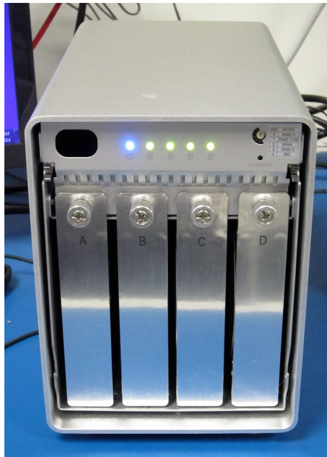
Fig. 10 Configurable four-drive RAID array with front panel removed.
