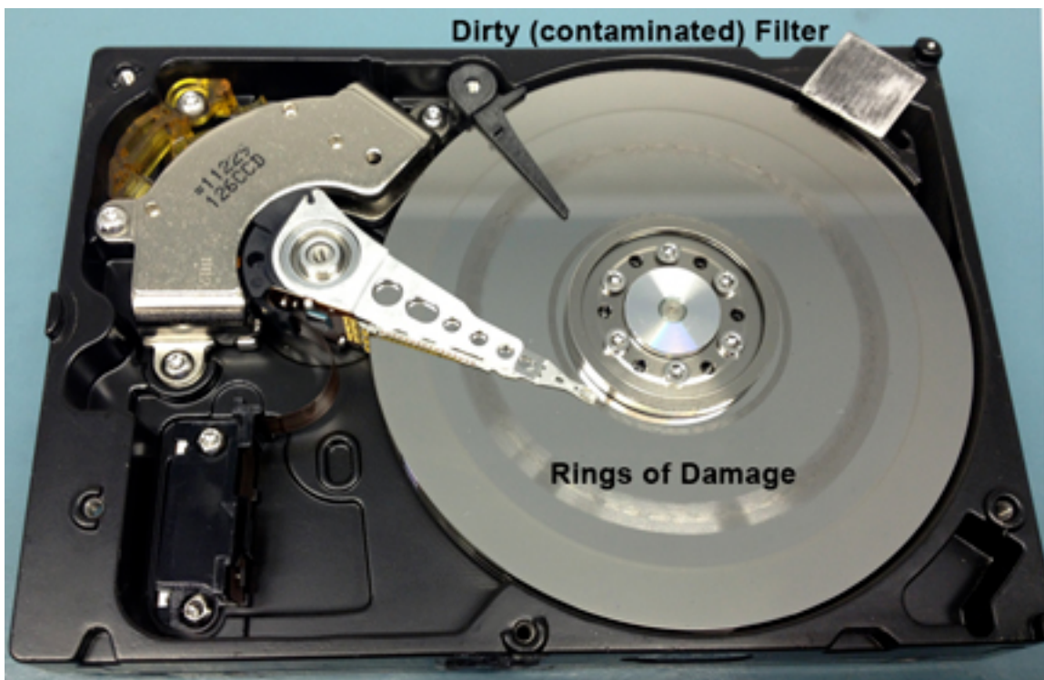
Fig. 7 A hard drive with a head crash and media damage.
