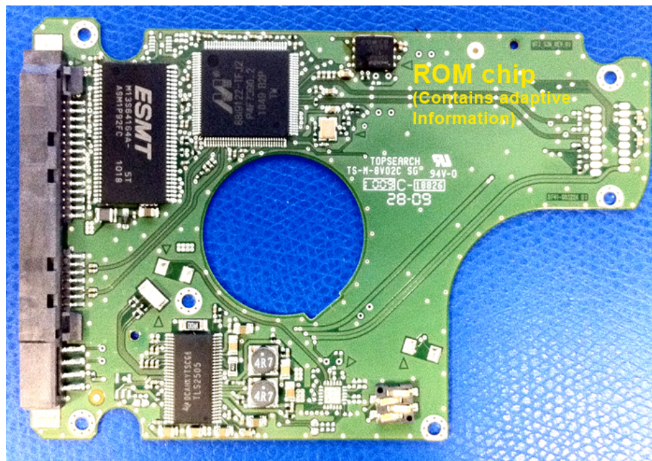
Fig. 4 A PCB showing a ROM chip .
