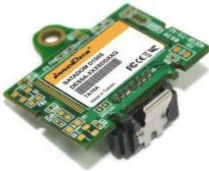
The SATA DOM device follows standard SATA electrical protocol on a custom connector. Unlike a standard SATA cable, it has a 5V power input to power the SATA DOM (as opposed to a SATA hard drive which has a separate power connector):
