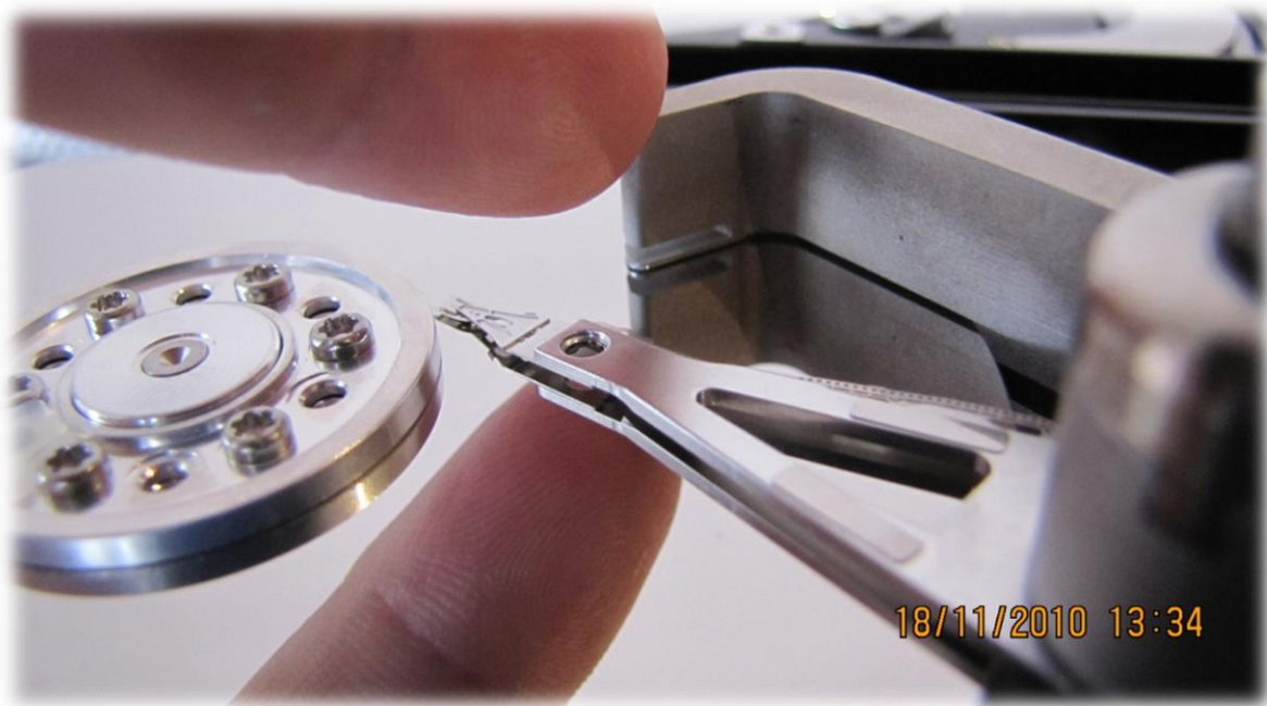
Picture 8. (returning the tool outside of platters)
